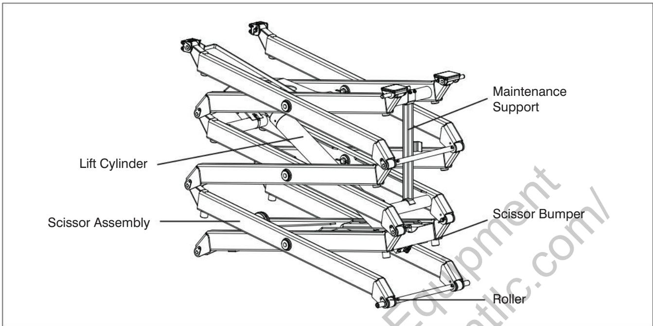
**2.3-9 Lifting Mechanism**
