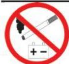
**Explosion hazard. Keep flames and sparks away. Do not smoke near batteries. Battery acid releases explosive gas while charging. Charge batteries in a well-ventilated area.**
