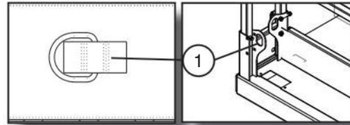
Figure 3-7. Fall Protection Anchorage
